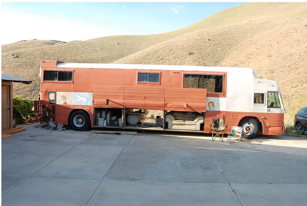
Turbo charged diesel pusher. Displacement 568 cu in (9.3 liters). Induction air intake is via scoop on roof.
